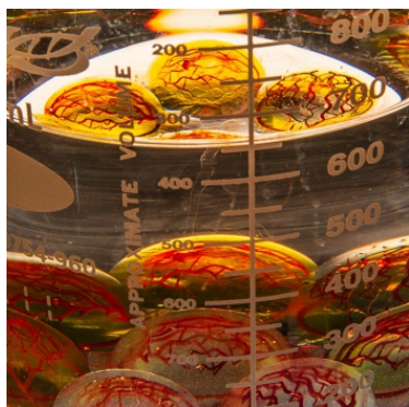
3D bioprinted soft tissue implant with vascularization channels perfused with red ink. The implant was printed using 3D Systems' high resolution stereolithography bioprinter and BioInk that is based on CollPlant's rhCollagen.
